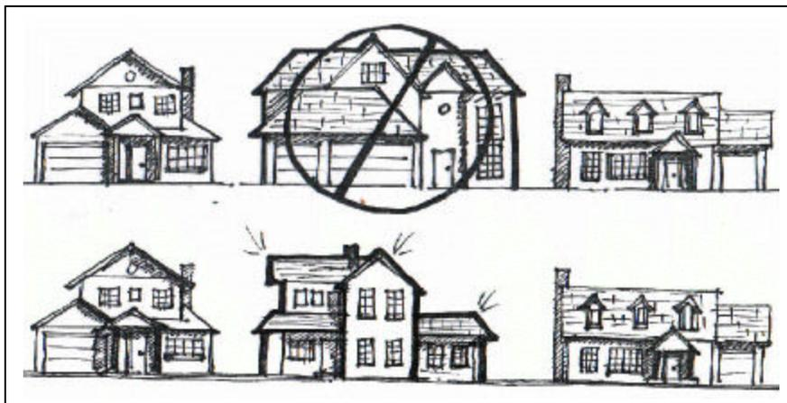
**The top sketch shows a new or remodeled home that does not fit. The bottom sketch shows how a larger home can be designed so as to fit into the neighborhood.**
